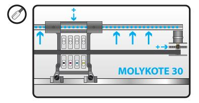
**Pour alcohol** (95% or higher) on a **cloth** and **clean** the **carriage shaft thoroughly**.
