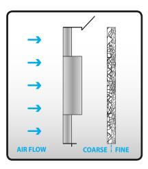
The fan filter collects the mist from the print head spray from the exhaust provided by the fan.
