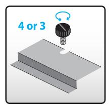
**Loosen** the four (or three, depending of model) black thumb **screws** (do not remove them completely) of the encoder cover, and remove the cover.
