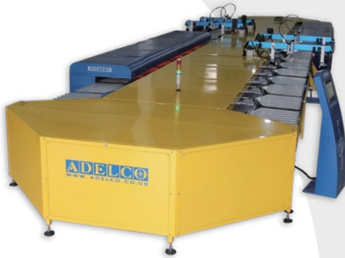
Bespoke oval design auto sock printer illustrated
